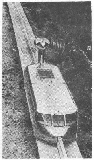
The Aerotrain, a rapid transit vehicle without wheels that could go from the Loop to O'Hare Airport in 10 minutes, according to its builders. France plans to put the Aerotrain into service on an experimental basis. The car, which rides on an air cushion along a concrete rail, was described to Chicago business at a conference on rapid transit systems.
